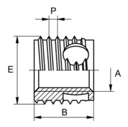
Female thread A = M3,5 Length B = 8 Male thread E = 6.0Min hole depth blind hole = 10
